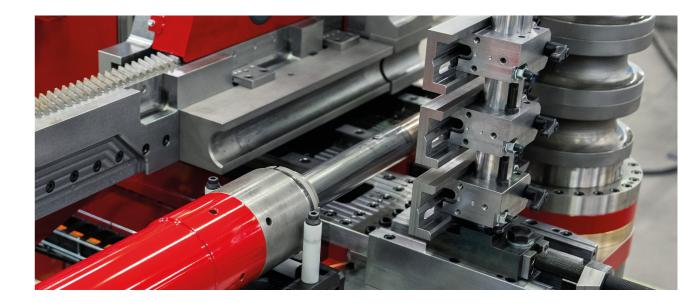
Herber is the inventor of boost tube technology, a widely used feature in the industry today. It allows tube bending without long straight end sections, eliminating the necessity for additional cutting. The boost tube technology streamlines the manufacturing process, reduces material waste, and enhances overall efficiency.
