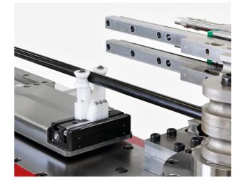
**Sometimes the simple things are the best.** Our programmable self-centering tube support allow you to have the support when you need it and out of the way in no-time.
