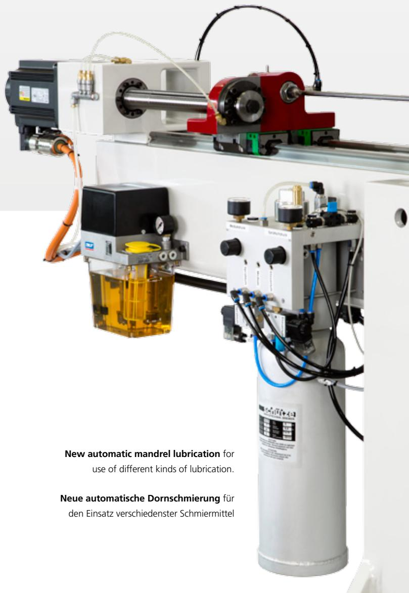
**New automatic mandrel lubrication** for use of different kinds of lubrication.
